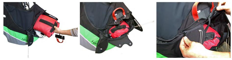
Take the bridle cover zip all the way to the right to then close it, moving the zip about 20 cm leftward. Then begin to close the various parachute container flaps, following the progressive order in the photographs, taking care during this phase that the zip does not open back up at the right end.
