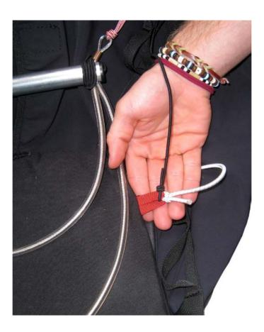
Then pass the last step inside the second step, so that the two are fastened to a degree. Twist the elastic cords previously tied to the base of the LEG COVER around the two steps of the speed system, as shown in the photo. Lastly, tie the elastic cord to the loops on the speed system.
