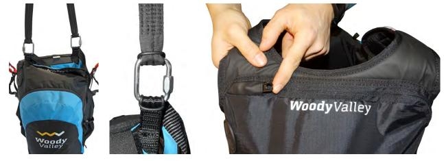
The two connections should be made using screw-lock karabiners with a breaking strength of at least 1,400 kg. It is important to verify that the length of the bridle is sufficient to position the reserve parachute inside the harness pocket, and that there is sufficient play to enable the parachute to be taken out of the pocket without causing the reserve parachute deployment bag itself to open during extraction.
